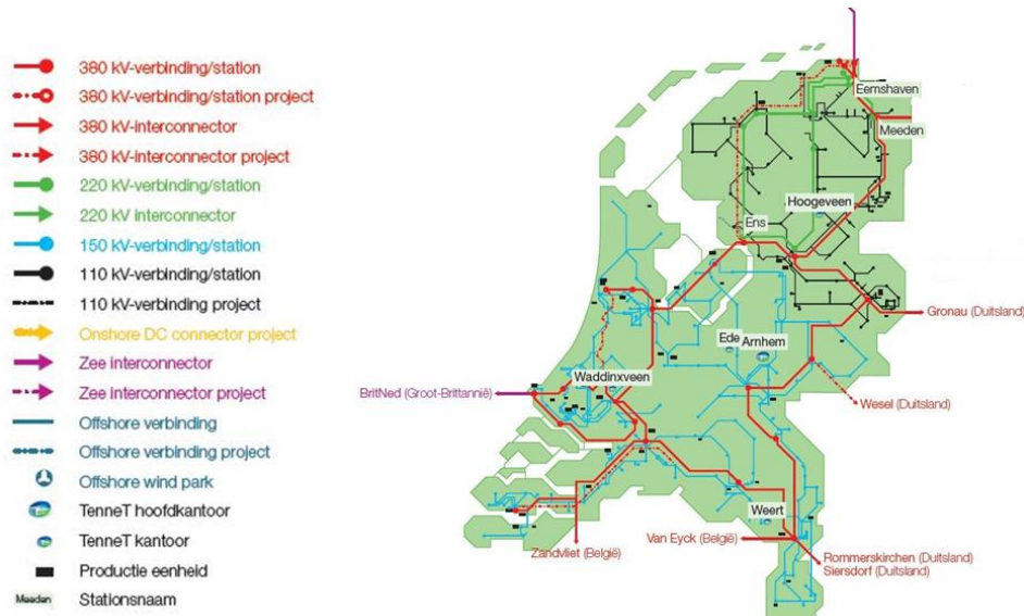
Figure 9. Electricity transmission grid in the Netherlands
