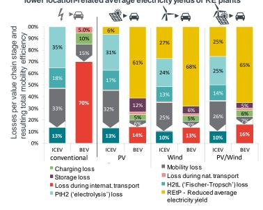
Electricity yield efficiency, i.e. capacity factor (here "reduced electricity generation yield"): Global best location for wind or PV = 100% (for details see section 3). PV - BEV: plants in Germany (DE); ICEV = plants in North Africa (NA); wind - BEV: plants in DE (onshore and offshore); ICEV: plants in Patagonia; PV/wind, 50% each - BEV: PV and wind plants in DE; ICEV: PV and wind plants in NA
