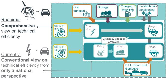
In a comprehensive assessment, PtL-powered ICEVs show similar efficiency to BEVs, especially since the importability of PtL products makes renewable energy sites with high electricity yield efficiencies usable
