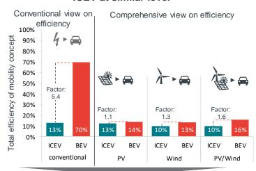
The main factor reducing efficiency in battery electric cars is the lower location-related average electricity yields of RE plants
