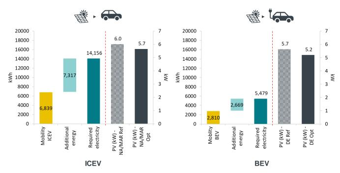
Note: **BEV - PV DE Ref**: PV generation in DE (969 FLH/ 39% yield efficiency), grid/transport losses: 5%, charging losses: 20%, storage losses (seasonal): 15%, efficiency BEV: 71%.
