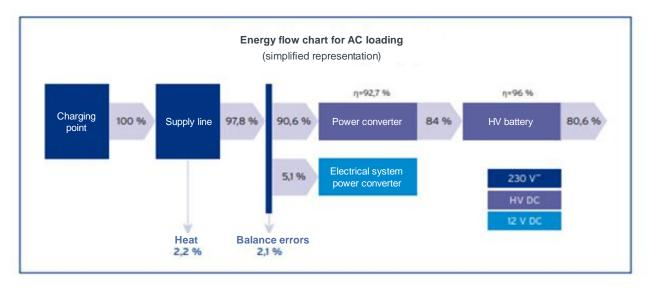
Figure 19. Example of charge losses during AC charging
