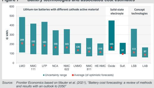
Figure 7 Battery technologies and associated cost estimates
