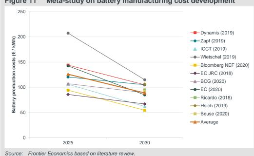
Figure 11 Meta-study on battery manufacturing cost development
