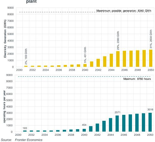
Figure 6 Electricity generation and operating hours of the 100% biomass plant
