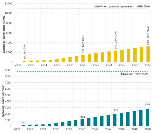
Figure 10 Electricity generation and operating hours of the combined biomass and hydrogen plant
